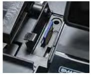
Secure SD Port SD Card Utilities include program Save/Load, report capture, firmware updates and graphics uploading.
